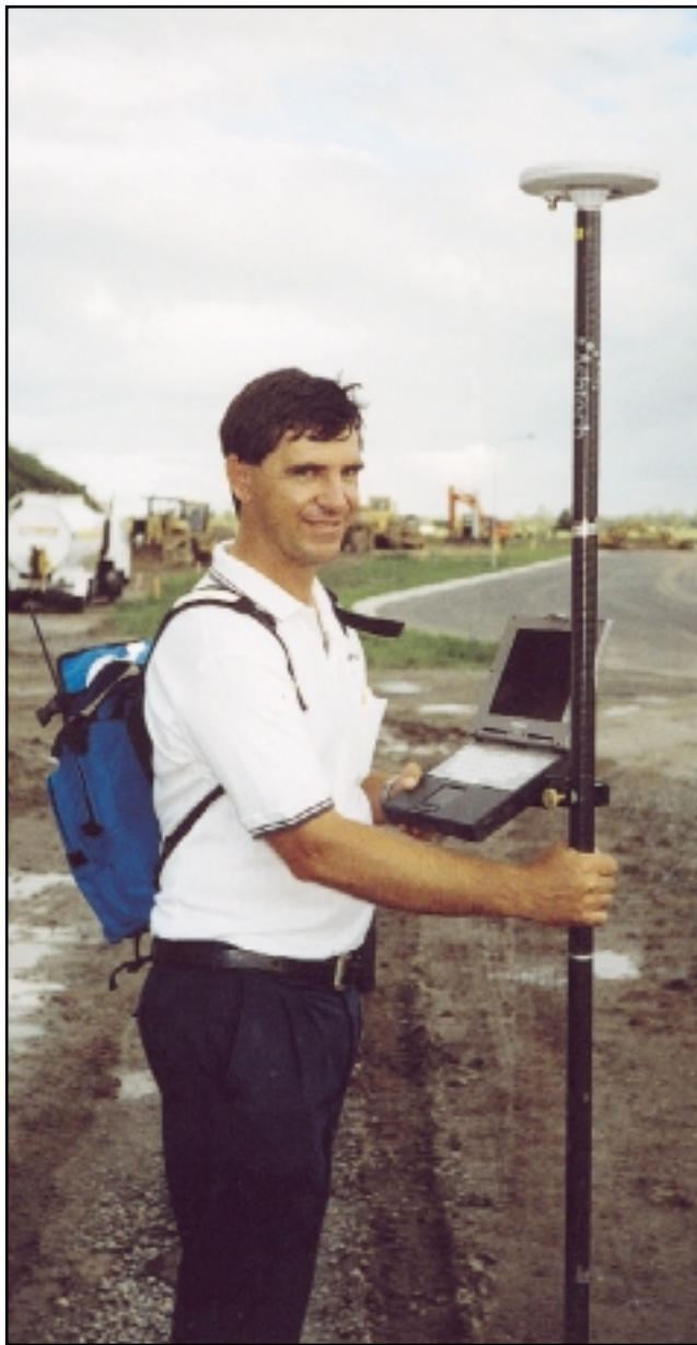
The GPS rover (above) has a convenient back pack. Computer is tiny— it attaches with a Velcro pad.
